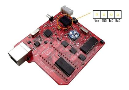
**Note**: the direction of the TX / RX lines is shown inverse, ie the way the pins of the Bluetooth module should be located. For example, Chinese HC-05 is directly compatible.
