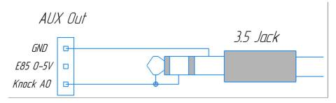
This output can also be connected to a recording device, such as a PC, to record the sound of the knock sensor signal through the microphone input.
