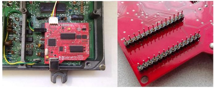
To ensure access to the CobraRTP USB port, it is necessary to make a cutout in the ECU case.
