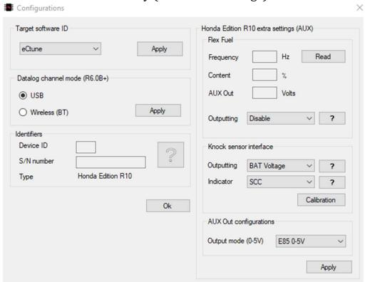
*Flex Fuel* – group of settings for the ethanol content sensor interface. Here you can check the current ethanol content readings and configure the *outputting* of the readings to the datalog channel data stream using the ISR protocol to indicate the ethanol content in HTS, eCtune, etc.
