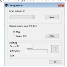
To switch the mode, you must select the appropriate item and save (the selected mode is saved in permanent memory).
