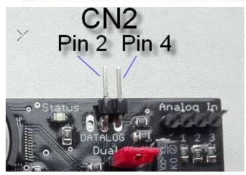
As you can see, two data lines are used for connection - RX and TX, respectively 2 and 4 pin of the **CN2** connector in the computer.
