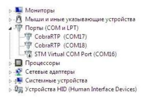
View of the device in the device manager upon successful installation of the driver (port numbers may differ from yours).
