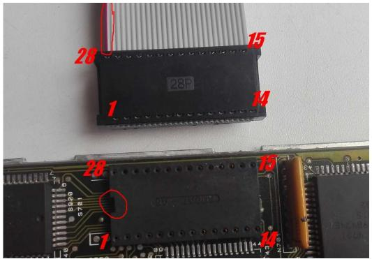
In all cases, it is necessary to navigate the red strip on the loop cable and the cutout on the socket, which should be on one side!
