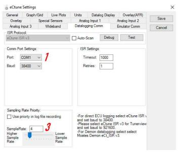
1. You must select the COM port number (see Connecting to a PC) for **Datalog** (**do not confuse it with the COM port number for emulation!**).
